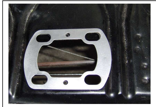
Thin steel shim on top of floor. It is often corroded. Replacement shim from vendors is plastic.
