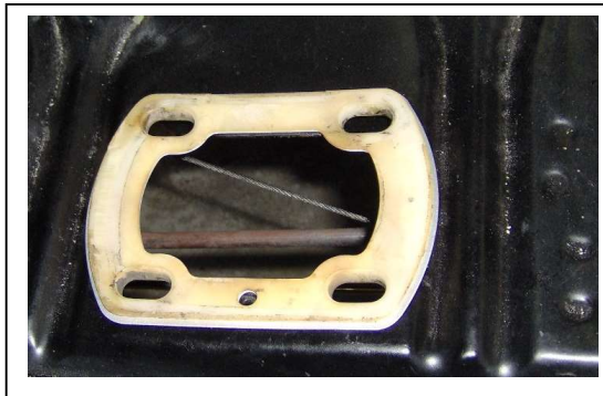
Plastic seal that sits on top of thin steel shim. Shifter lever and base sit on top of seal.
