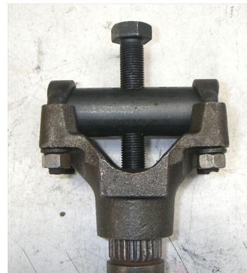
Yoke Puller installed for use On 1960-64 Axle
