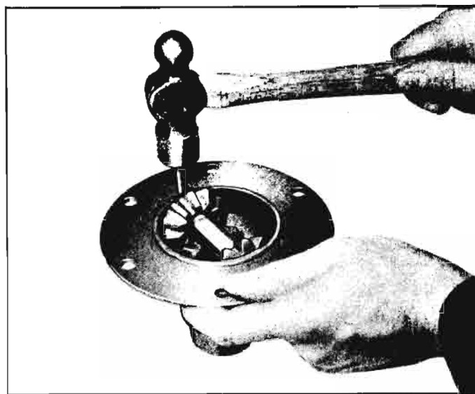
Fig. 6C-35—Installing Pinion Shaft Pin
