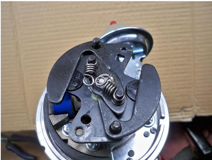
5) Rotate distributor to horizontal in vise, sticking out the side
