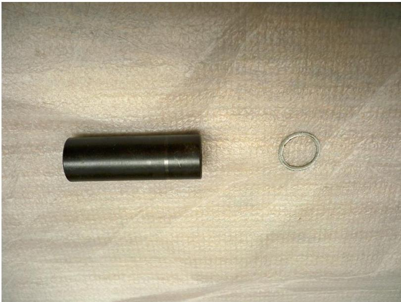
The tubular spacer also acts to protect the feed wires from rubbing on the distributor shaft when it is in operation. With the main shaft removed, the reluctor assembly is free to slide down the shaft and be removed – unless you have let the two advance weights in place. Those will keep them together.
