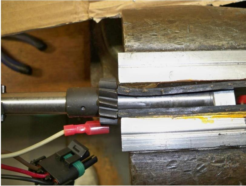
6) Remove retainer nut for advance sleeve – 7mm open end wrench
