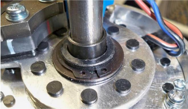
6) Center the spacer and re-install the snap ring to retain the rotating plate. Make sure the spacer has fully dropped into place and the snap ring is fully in the slot.
