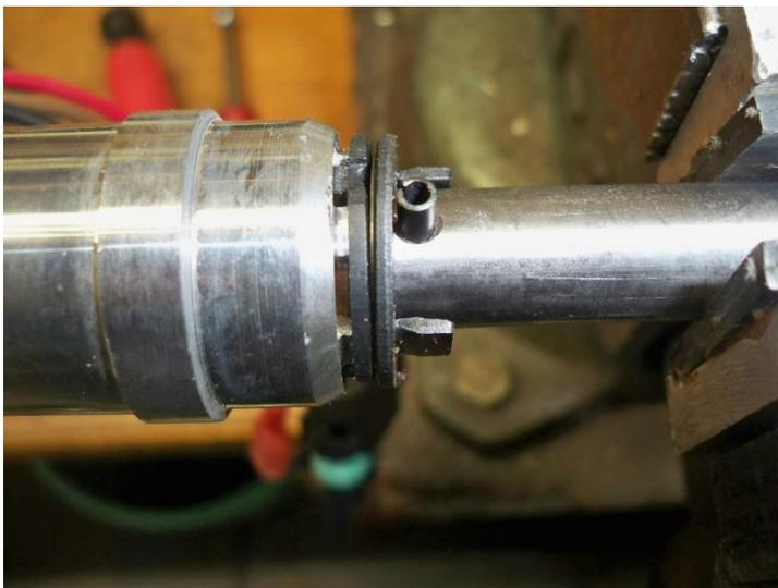
3) Slide the main shaft out the top with the reluctor still in place. Be sure to note the location of any spacers on the shaft, they need to go back in place. Note where the interference is – usually on the outside of the slot.
