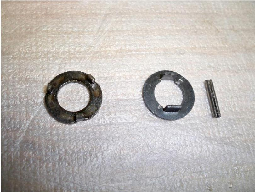
At this point the main shaft, along with the reluctor, may be withdrawn from housing. There will be one or two spacers on this shaft, one long, tubular one and one thin washer-style one. They should stay on the shaft as it is removed, but might remain in the distributor.
