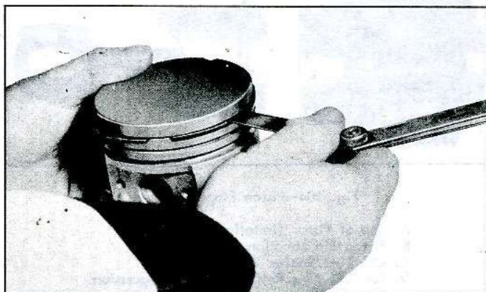
Fig. 106—Measuring Ring Groove Clearance
