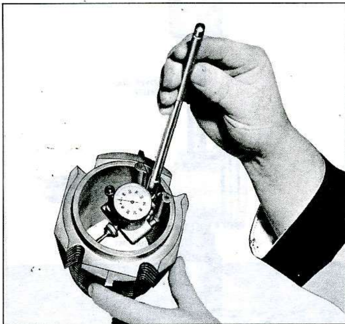
Fig. 100—Measuring Cylinder Bore
