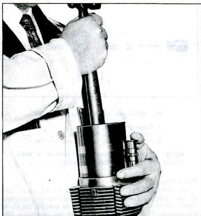
Fig. 107—Installing Piston in Cylinder
