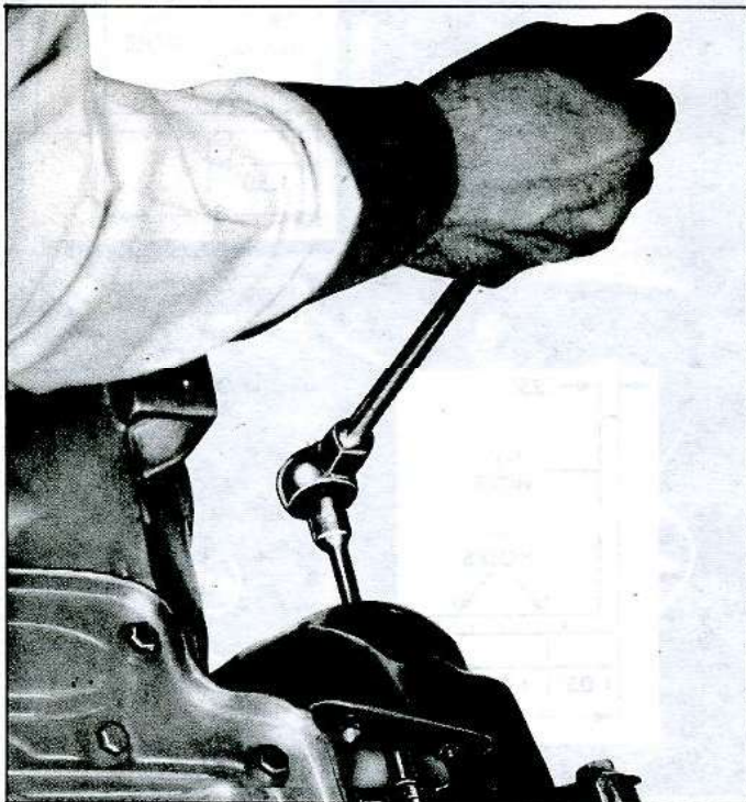
Fig. 51—Removing Left Front Shroud
