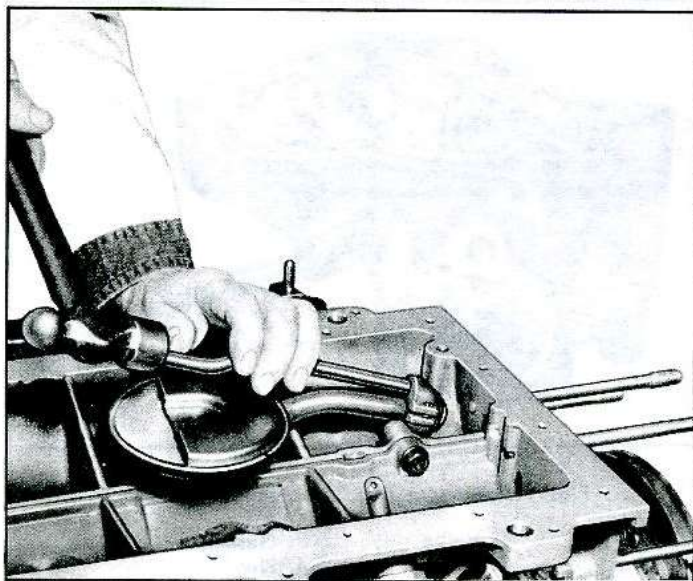
Fig. 108—Installing Pick-Up Screen and Tube
