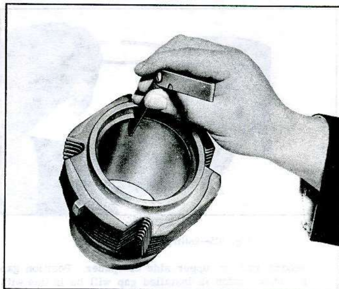
Fig. 103—Measuring Ring Gap
