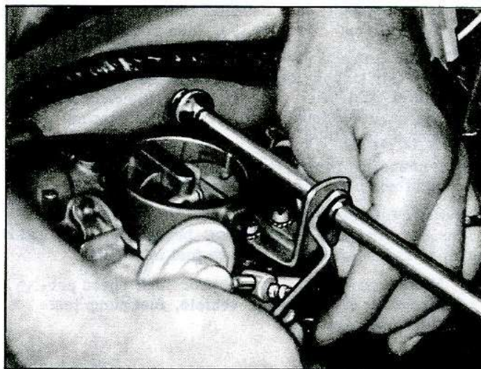
Fig. 9—Adjusting Accelerator Rod
