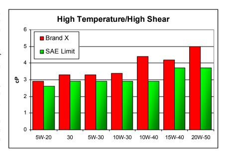
In this example, the Brand X 10W-40 is synthetic. It therefore behaves like a SAE 40 under stress.
