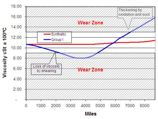
In engines that depend on gears for timing (rather than timing belts and chains) there is often a tendency to shear at a very high rate. This is not as big a problem in Corvairs because the timing gears are larger in diameter, slowing their contact and milling action.
