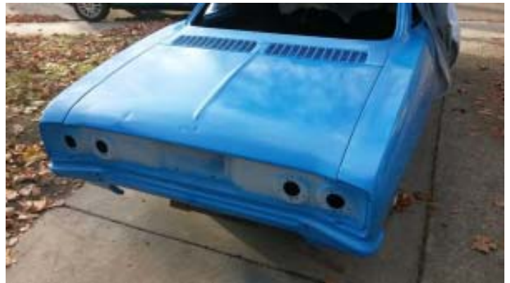
Rear deck painted. Dents won't matter as they will be covered by the Tin Tail spoiler.
