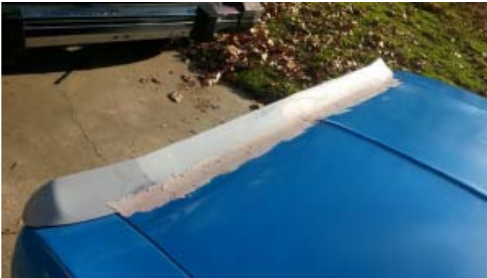
Tin Tail primed, installed and puttied. Ready for final sanding and paint.
