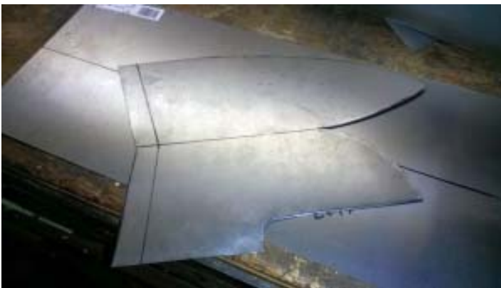
Tin Tail parts being cut out. Done in several pieces because Steve's break not large enough.
