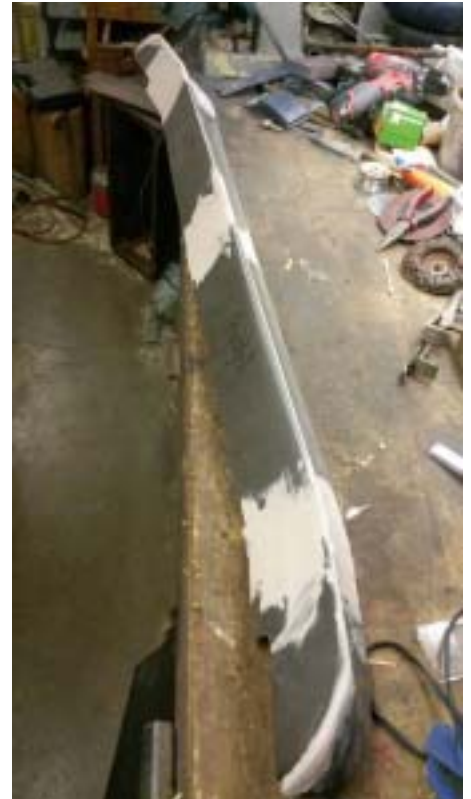
Final assembly after welding, grinding & filling. Body putty was used to get a final smooth shape. This has been sanded and is ready for priming and painting.
