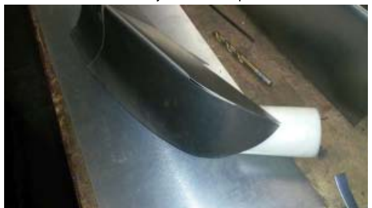
End piece bent into shape. Ready for welding and finishing.
