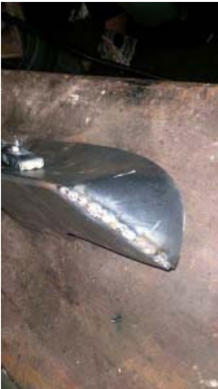
Tin Tail parts being cut out. Done in several pieces because Steve's break not large enough.
