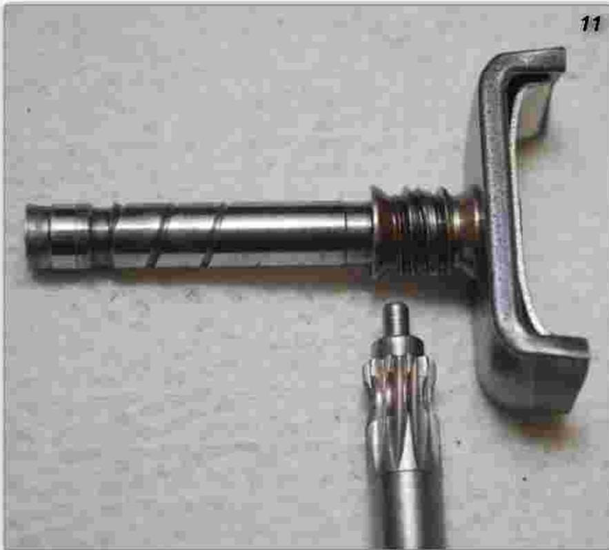
on the other end of the shaft with a small diameter pin and the entire bushing and shaft will pop out. Once out, clean and inspect the diagonal gear shaft and the worm gear below the spinning magnet.
