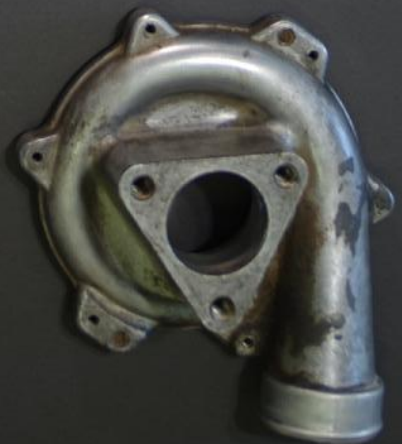
A Corvair 'F' Flow Cover, Machined to take the 'E' Flow Compressor Wheel
