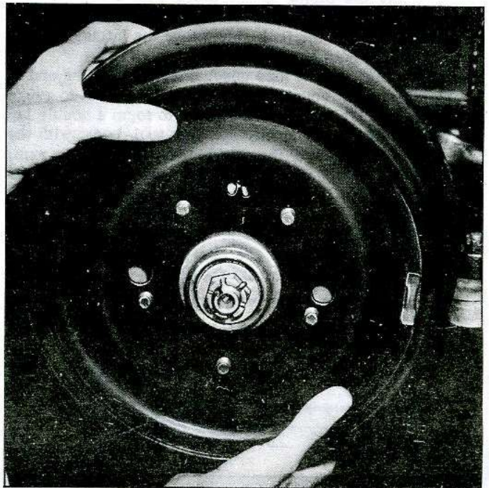
Fig. 15—Aligning Drum Tang with Wheel Hub
