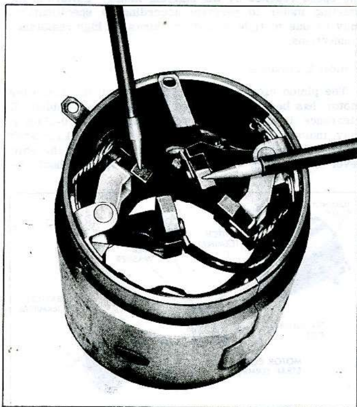
Fig. 8s—Field Coil Ground Test
