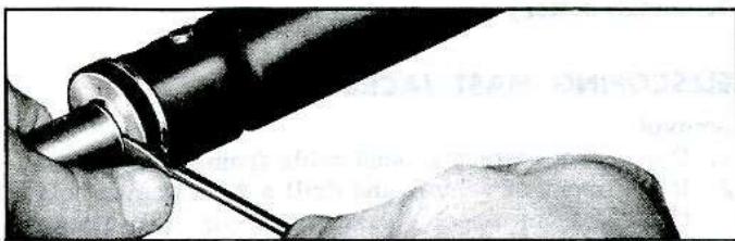
Fig. 20—Removing Lower Snap Ring
