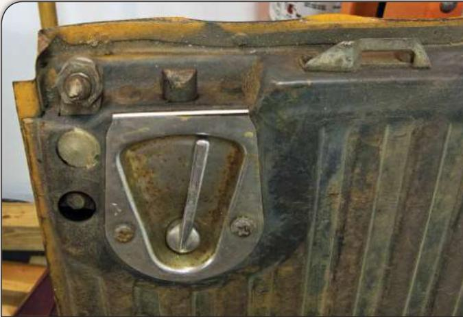
When restoring the ramp, which had to be disassembled, precise alignment of the guiding pin was critical, as the closed ramp provides an important structural component for the bed that would otherwise flex substantially when the pickup was moving.
