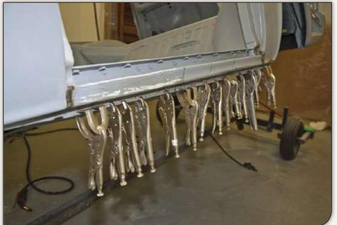
The Rampside's unique, mid-bed door gave the chassis an obvious weak point, the rocker panel essentially the only structure holding it together. More than a dozen locking pliers were required to keep the piece straight when welding it back together.
