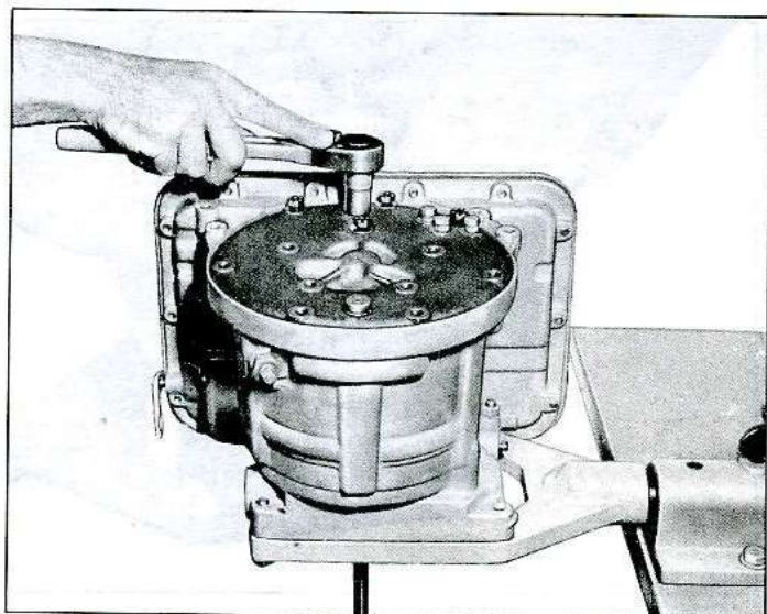
Fig. 7E-18—Removing Front Pump Bolts
