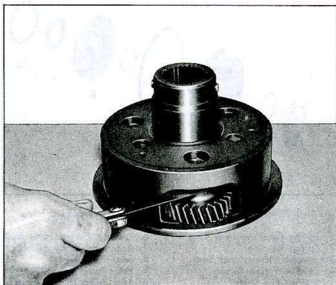
Fig. 7E-44—Checking Planet Gear End Clearance
