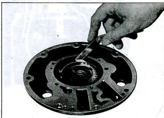
Fig. 7E-32—Checking Driven Gear-to-Crescent Clearance
