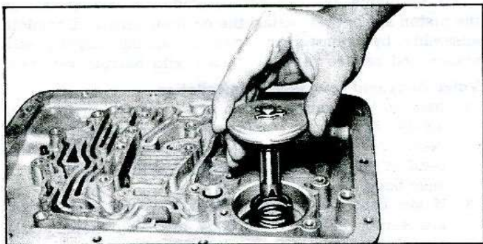
Fig. 7E-14—Installing Low Servo Piston and Return Spring
