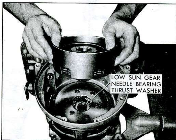
Fig. 7E-23—Removing Clutch Drum
