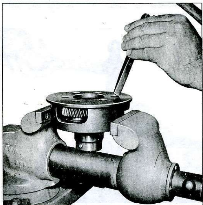
Fig. 7E-48—Staking Planet Pinion Shaft
