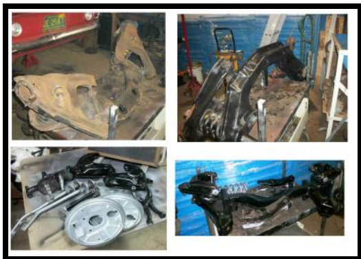
Figure 8 Rebuilding the suspension
