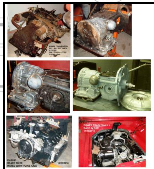
Figure 3 The power train was a mess - we did get it running before removing from car but the engine knocked so we replaced it with a used engine.
