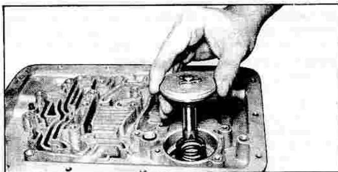
Fig. 7E-14—Installing Low Servo Piston and Return Spring
