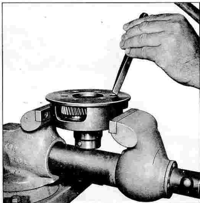
Fig. 7E-48—Staking Planet Pinion Shaft
