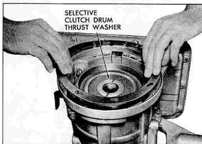
Fig. 7E-57—Installing Front Pump Gasket
