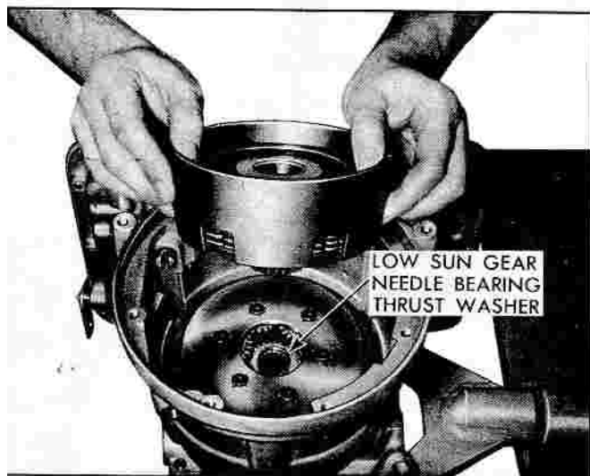
Fig. 7E-23—Removing Clutch Drum
