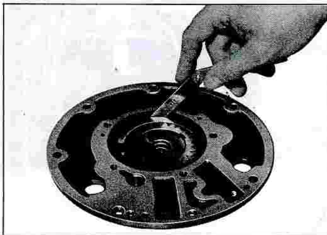
Fig. 7E-32—Checking Driven Gear-to-Crescent Clearance
