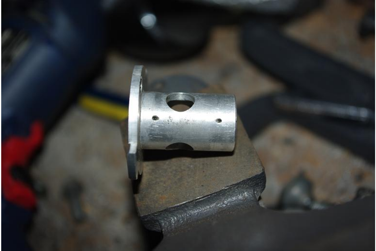
A side view of the same bearing. Large holes are oil drains, small ones are the direct feeds to the journals.
